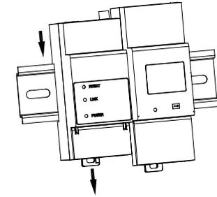
Fig 3.1 Installation method
